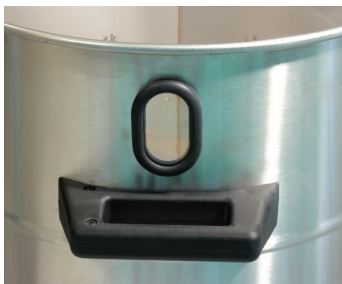
Sight Glass on Recovery Tank
