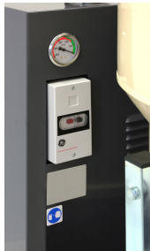
Planet 775 Filter Blockage Indicator Gage. Manual Starter with Overload Protection
